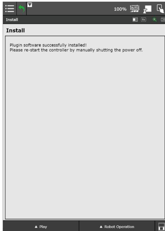
After the prompt to restart the robot controller, switch it off at the main switch and switch it on again after about ten seconds. The teach pendant does not have to be restarted. Wait until the teach pendant has re-connected with the robot controller.
