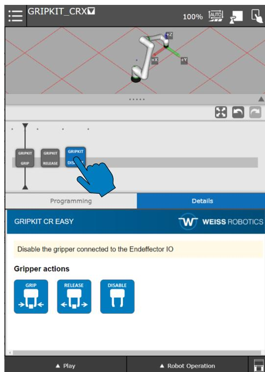
Alternatively, the actions can be performed as a call of the corresponding TP program. To do this, the respective program must be selected in the TP editor using "NEW INSTRUCTION", "CALL", "CALL program". The TP
