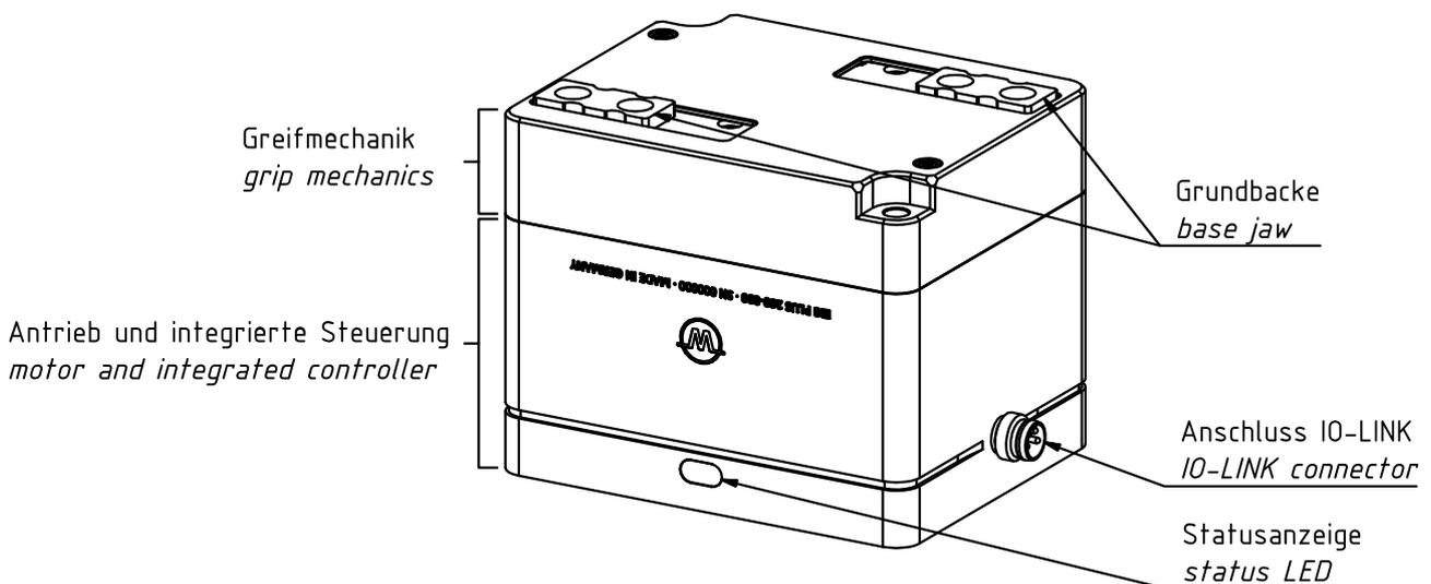
Figure 1: Components and connectors of the gripping module
