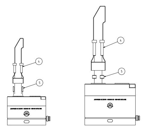
Figure 8: Mounting the fingers
