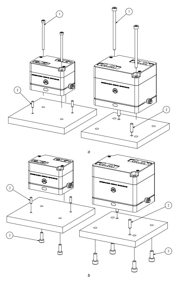
Figure 7: Mounting methods for the gripping module from above (a) and from below (b)
