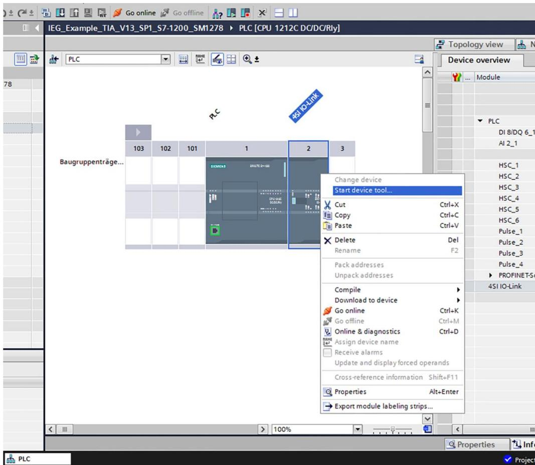
Figure 24: Starting the S7-PCT port configurator (device tool)
