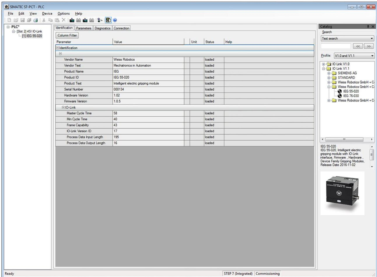
Figure 26: Identification of the gripping module in S7-PCT
