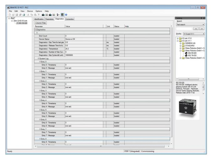
Figure 28: Diagnostics data of the gripping module in S7-PCT
