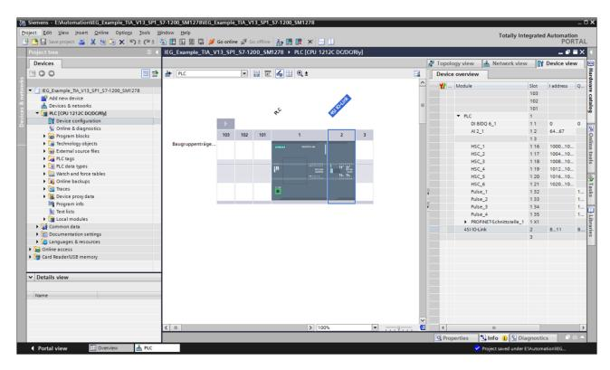
Figure 23: Configuration of the IO-Link master
