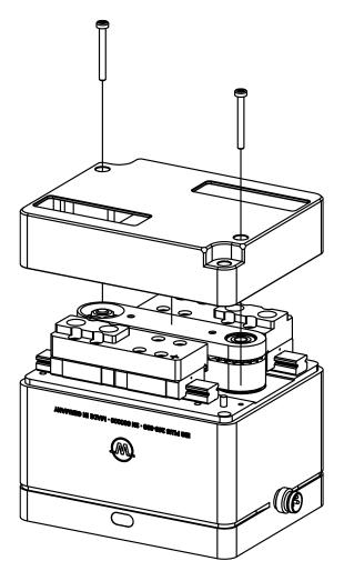
Figure 22: Removing the belt cover
