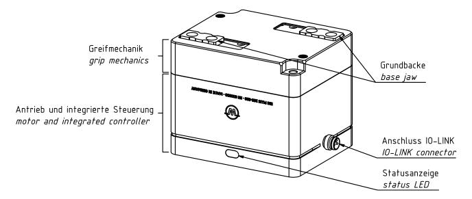
Figure 1: Components and connectors of the gripping module
