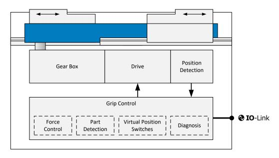
Figure 9: Functional diagram of the IEG PLUS gripping module
