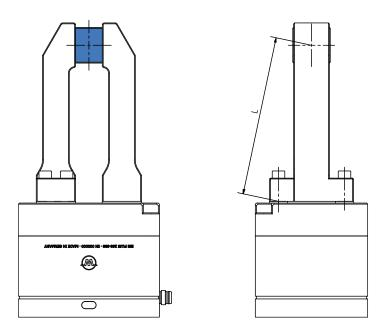
Figure 2: Determination of the finger length "L"
