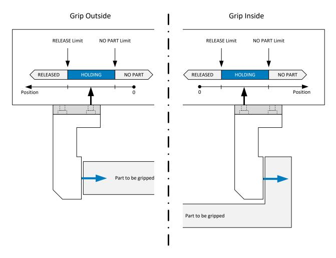
Figure 14: Gripping area and gripping direction
