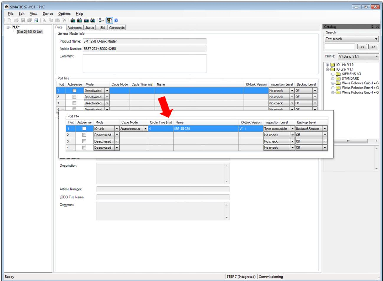
Figure 25: Configuration of the IO-Link port
