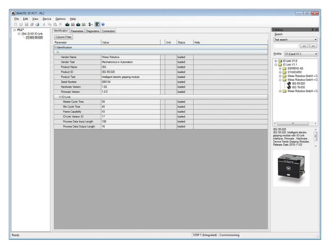
Figure 26: Identification of the gripping module in S7-PCT
