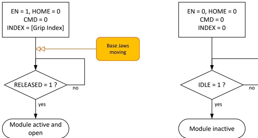
Figure 19: Program sequence to activate (left) and deactivate (right) gripping module
