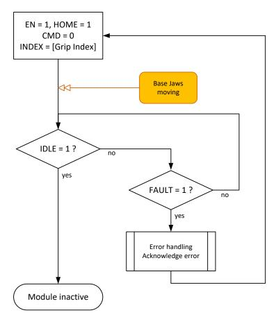
Figure 15: Initializing the gripping module
