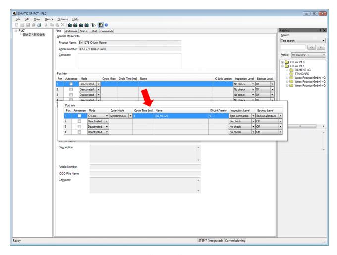
Figure 25: Configuration of the IO-Link port
