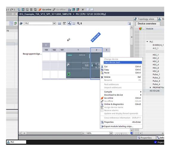
Figure 24: Starting the S7-PCT port configurator (device tool)
