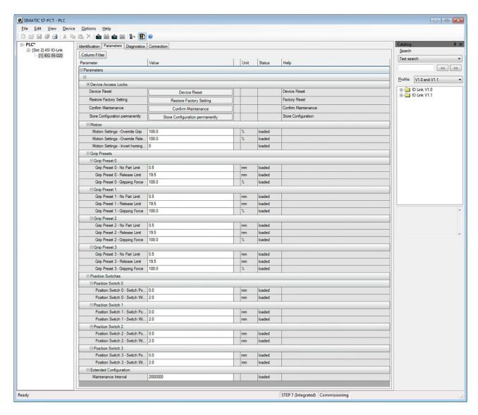
Figure 27: Parameters of the gripping module in S7-PCT
