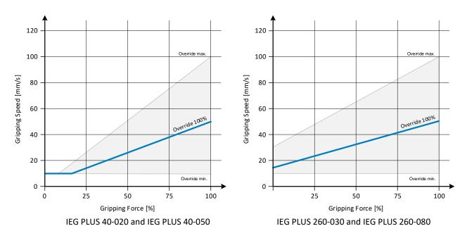
Figure 3: Gripping speed depending on the parameterized gripping force
