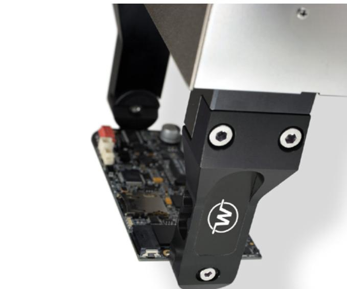
*Sensor fingers with interchangeable pads and integrated force sensing for WSG 32 and WSG 50 enabling precise and dynamic grip control, increased process reliability, and optimal handling of sensitive parts.*
