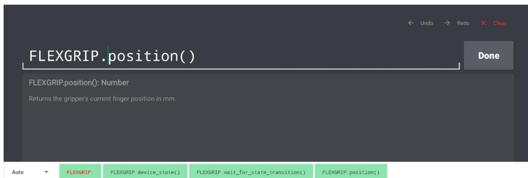
The screenshot shows a function call editor for `FLEXGRIP.position()`. The function signature is `FLEXGRIP.position(): Number`. The description states: "Returns the gripper's current finger position in mm." Below the editor, a list of available functions is shown:
