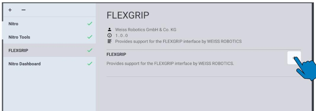
A new instance now appears in the device list. If several grippers have been created, a number is added, e.g. “FLEXGRIP2”. Errors are still displayed here as the configuration has not yet been completed (refer to section 4.2).
