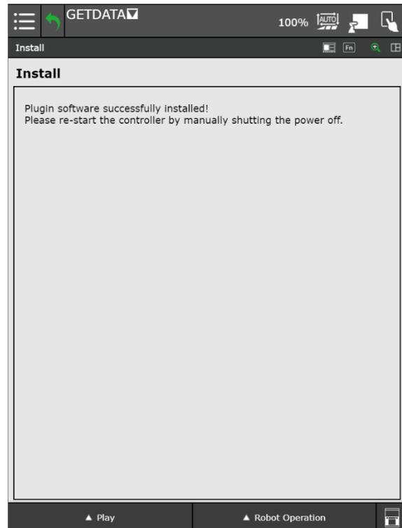
After the prompt to restart the robot controller, turn off the mains switch and back on again after ten seconds. Alternatively, the restart function on the teach pendant can be used (refer to the robot controller’s manual for further information). Restarting the Tablet Teach Pendant is not required. Wait until tablet and robot controller reconnected.
