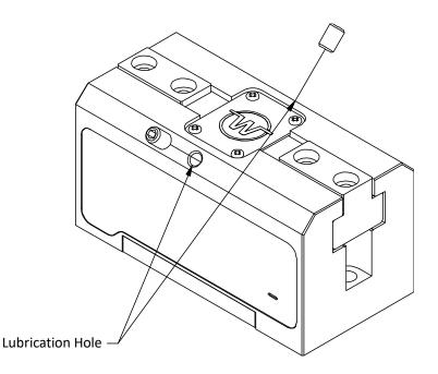
Figure 25: Position of the lubrication holes
