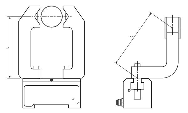
Figure 2: Determination of the finger length "L". Left: straight fingers, right: angled fingers
