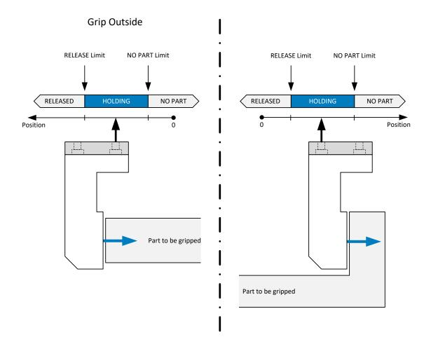
Figure 15: Gripping area and gripping direction
