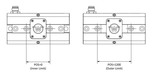
The integrated position sensors are not designed for measurement tasks.
