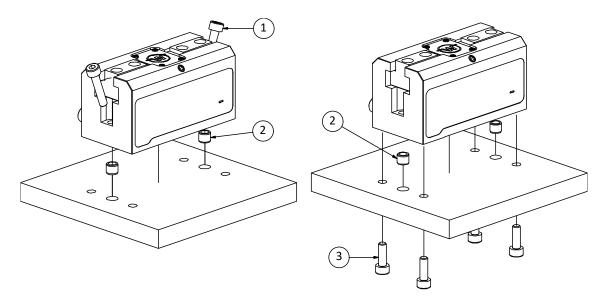
Figure 7: Mounting methods for the gripping module
