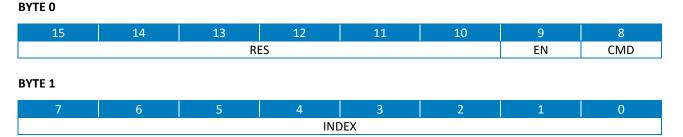
Table 8: Process data word IO-Link master to gripping module
