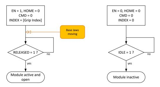
Figure 20: Program sequence activating (left) and deactivating (right) gripping module
