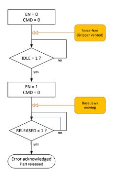
Figure 19: Program sequence acknowledging an error and releasing a part
