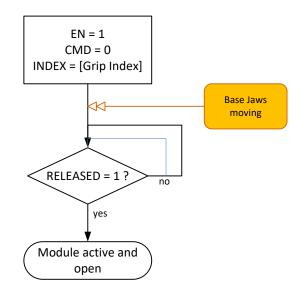
Figure 16: Program sequence activating the gripping module
