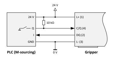
Figure 24: Connection to M-sourcing PLC in SIO mode
