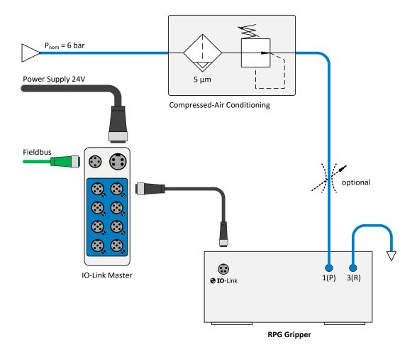
Figure 10: Connecting the gripping module
