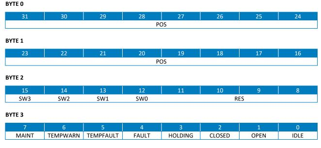
Table 9: Process data word gripping module to IO-Link master
