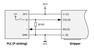
Figure 23: Connection to P-sinking PLC in SIO mode
