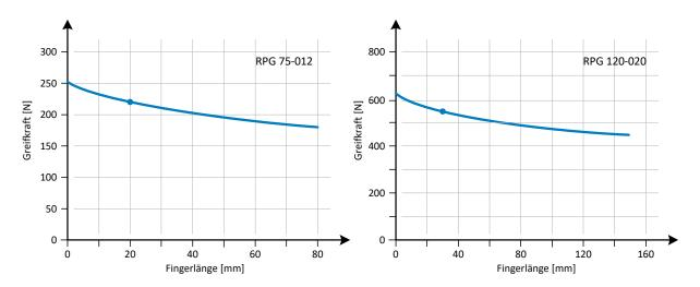
Figure 3: Gripping force diagrams with P<sub>nom</sub> = 6 bar
