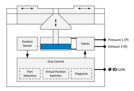
Figure 11: Functional diagram of the RPG gripping module
