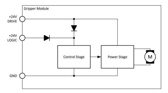
Figure 14: Equivalent circuit for the power supply
