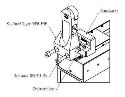
Figure 17: Installation of the fingers
