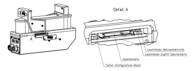
Figure 20: Tray to access the control unit
