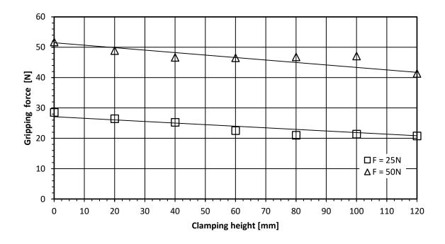
Figure 7: Gripping force over clamping height diagram
