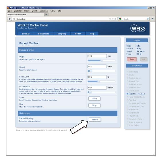
Figure 19: "Manual Control" configuration page
