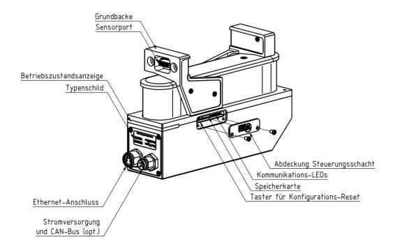
Figure 1: Components and connectors of the WSG 32
