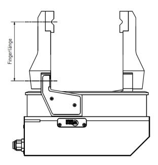
Figure 3: Determining the clamping height
