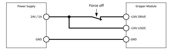
Figure 16: Connection type: Supply to load separate from supply to logic
