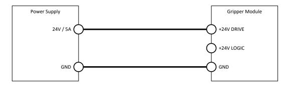
Figure 15: Connection type common supply to load and logic
