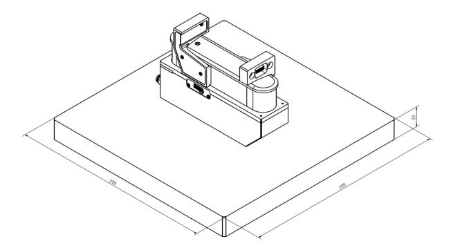
Figure 8: Arrangement for ascertaining the nominal gripping force
