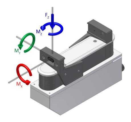
Figure 5: Mechanical finger load
