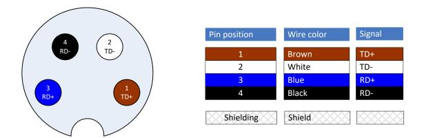
Figure 10: Pin assignment of the Ethernet connector (view on the socket).
