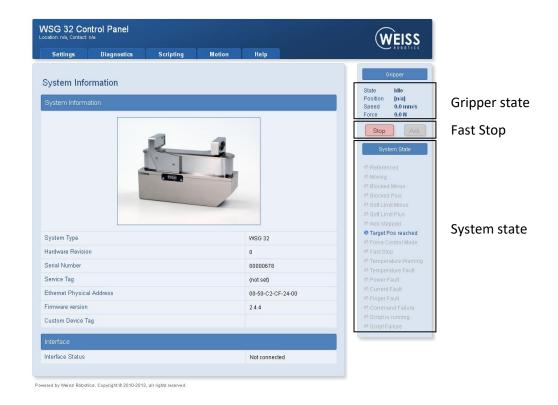
Figure 22: Web Interface side bar with system state
