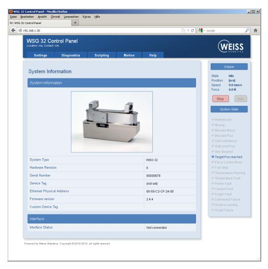
Figure 18: The starting page of the web-based interface
