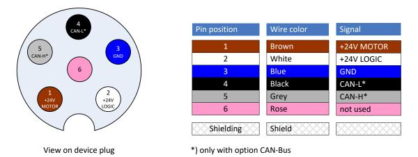
Figure 9: Terminal assignment of the power supply and CAN-Bus connector
