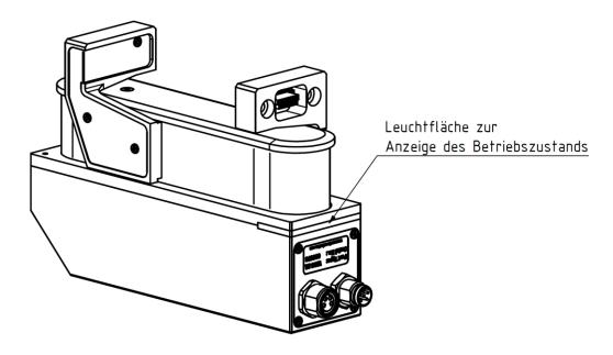
Figure 21: Display of operating state
